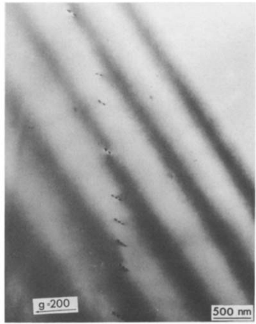
Figure 5 Bright-field TEM of the \{110\}\langle 110\rangle slip system together with another slip system, possibly \{111\}\langle 110\rangle . The dislocations have a mixed screw/edge character. The specimen is \text{TiC}_{0.79} deformed with a Vickers diamond. The foil normal is \langle 100\rangle .
